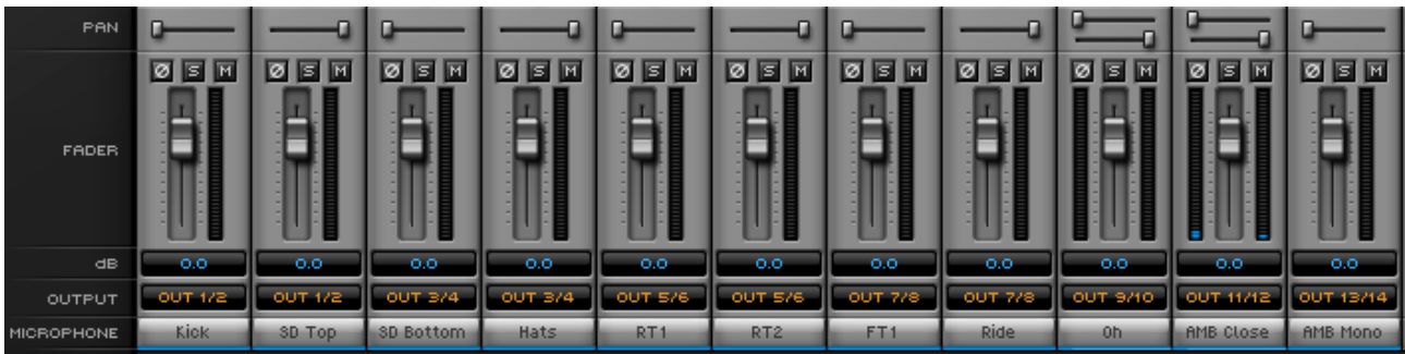
(Fig.4 - Superior Drummer stereo outputs. Pan hard to rout signal to mono side in sequencer)
