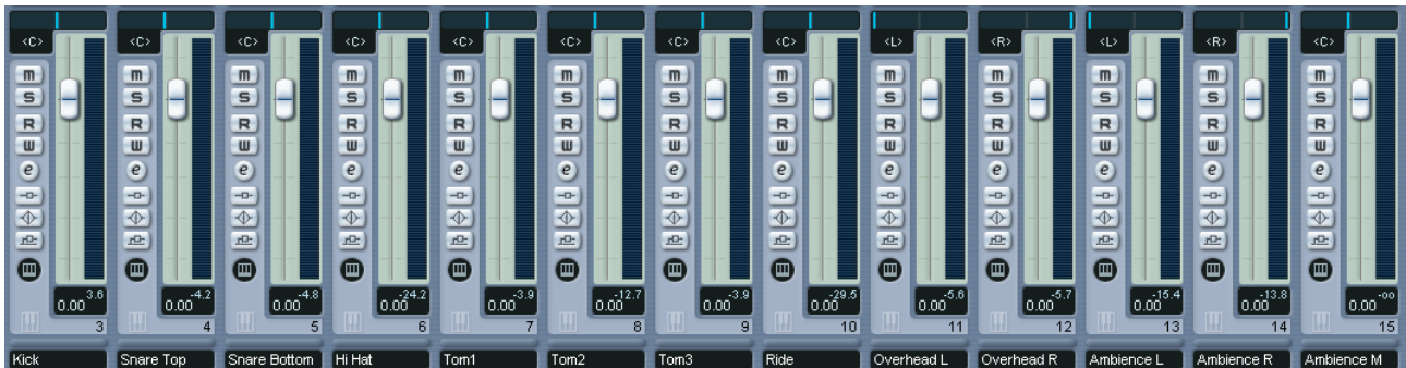
(Fig.5 - Superior Drummer stereo outputs into mixer showing as individual left and right)
